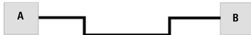
Figure 3 Straight pipe routing between two buildings, with expansion accommodated by Z-bends within the pipeline.
